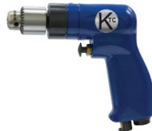
The KAT112 is a small, lightweight Pistol grip air drill with plenty of power. Designed to fit in the palm of your hand. High quality, designed for professional use. Features include progressive throttle, rotatable rear exhaust, 1/4" air inlet, 3/8" x 24 threaded spindle, 1/4" chuck and key, smooth quiet operation and one-year warranty.
