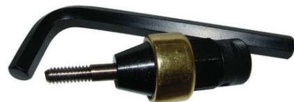
The KTC Wrench Style Rivnut tool is ideal for occasional or limited use. Will also let you apply more pull-up force than is generally available from the lever type rivnut tool. Hold the body with a wrench and turn the pull-up stud with the supplied wrench. Metric sizes indicated by \*.
