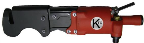
The KAT351PU Pneumatic Roof Punch is designed to punch a clean, burr free hole that is much faster and cleaner than drilling. The pneumatic punch delivers 5,400 lbs. of force, which provides enough power to punch through 3/16" thick material. It has a 1-7/8" reach and a 1/2" gap. 21" overall length. Specify punch and dies when ordering. Created for the semi-truck trailer industry for punching roof rail holes rather than drilling.
