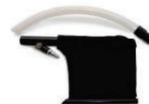
The KTC565 Aluminum Mini Vacuum is designed as a small light weight tool with plenty of power. Vacuum uses 90 to 120 psi and creates enough vacuum to pick up nuts, bolts, rivets, chips, dust etc. A great shop tool as well as a handy vacuum to clean up in the cock pit or in other confined areas 1/4" air inlet.
